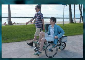
The Cycling Wheelchair (CW) is a pedal-driven wheelchair enabling even people who have lower limb disabilities to move it with their own leg strength. By controlling the brake and the Continuous Variable Transmission (GVT) attached to the wheels, we have realized many assistive functions. This wheelchair was demonstrated at the Honolulu Marathon several years ago.
