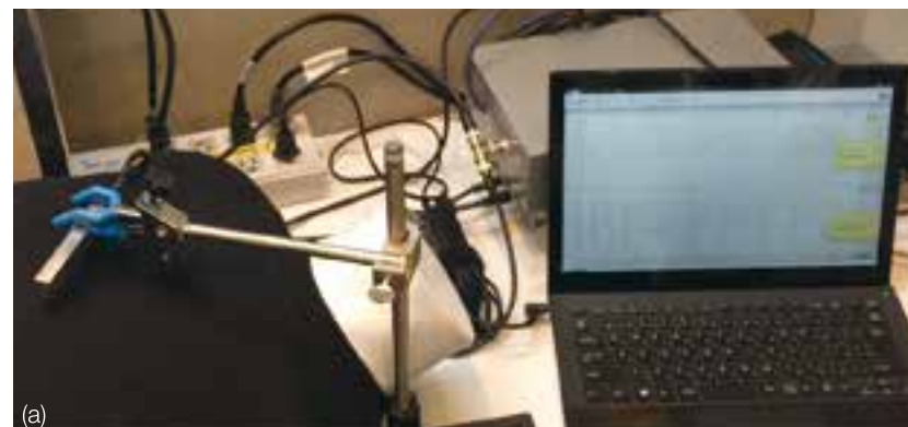
(a)MCG system with a sensor module and measurement system. The sensor module is set on a mannequin and detects an electrocardiogram (ECG) and MCG, simultaneously. (b) Electric circuit with TMR sensor inside the module. (c)ECG signal (upper) and MCG signal (lower) on the Monitor.
