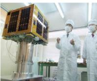
Recently our second micro-satellite RISING-2 entered into orbit at 628km altitude by the Japanese H-IIA rocket, on May 24, 2014. A month later, color images of the Earth surface were observed at about 5m spatial resolution by utilizing the High Precision Telescope (HPT). This spatial resolution holds the world record in the under-50kg category for micro-satellites. HPT can observe multi-spectrum images selected
